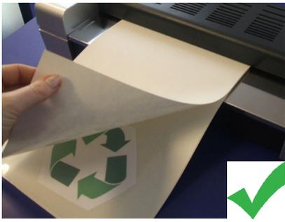
Never laminate without using a Lifejacket® or card carrier or you risk jamming and damaging your laminator (this will not be covered under warranty)
